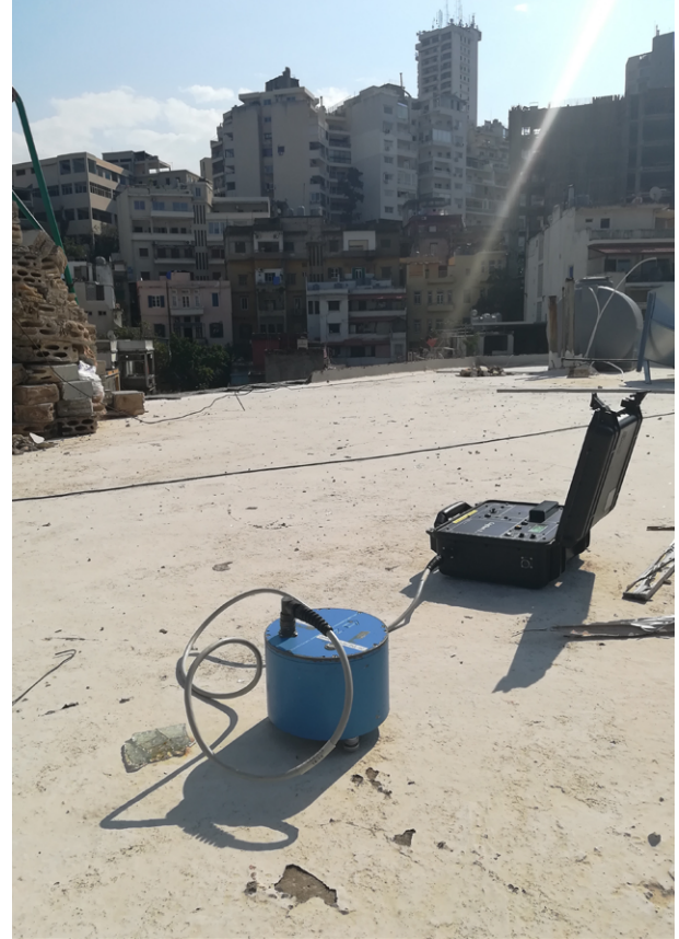
→ Acquisition system (CityShark TM and Lennartz 5s) used to measure ambient vibration in damaged buildings in Beirut, following the explosion of 4 August 2020. © C. Cornou, IRD/ISTERre
